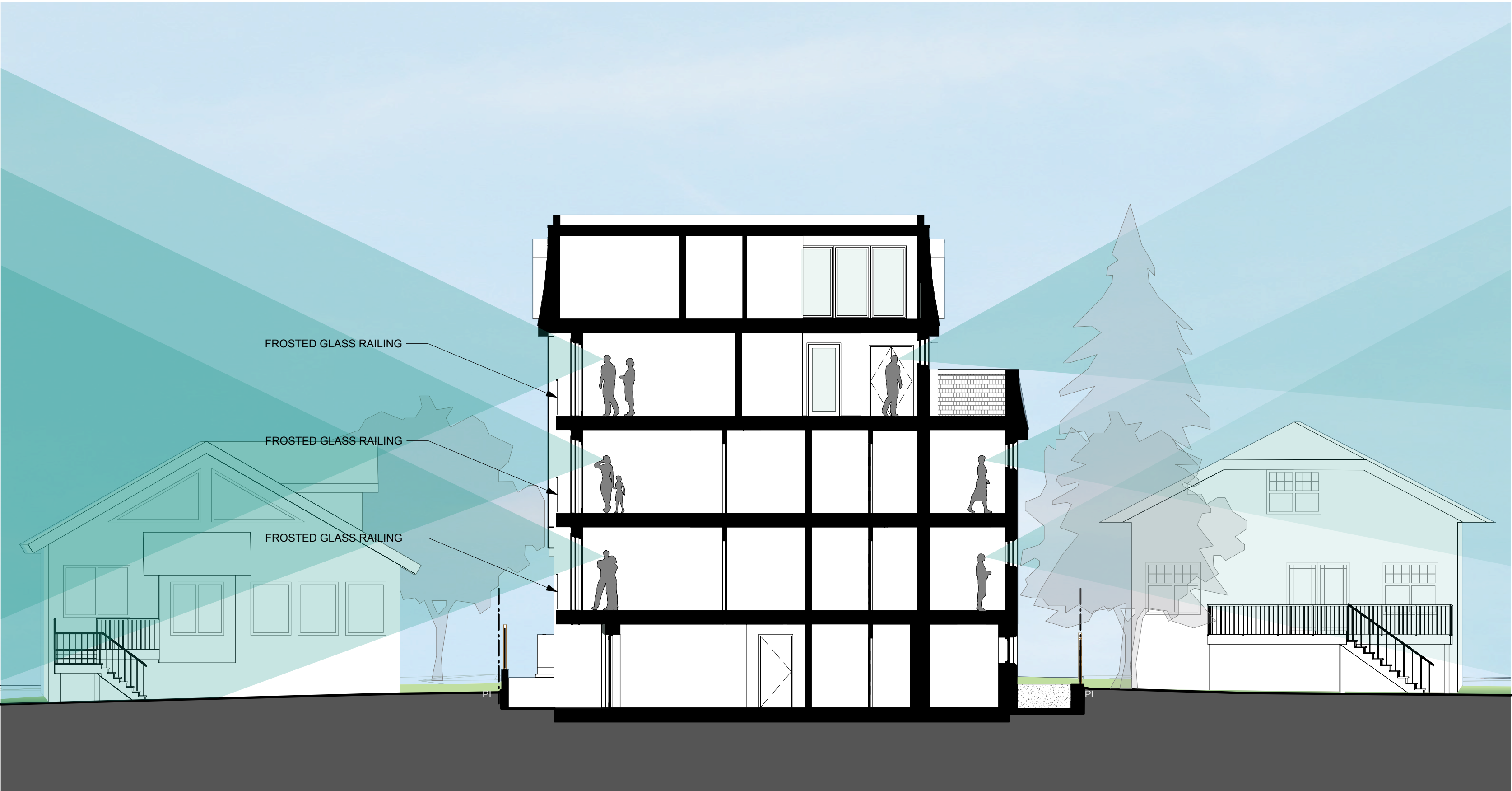
1 Sightlines (Section) RZ-302 Scale: 1:100
