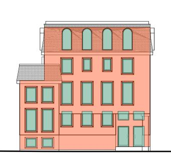
Table 3.2.3.1-D, BCBC LIMITING DISTANCE = 10.08m PROPOSED UNPROTECTED AREA = 48.38 m<sup>2</sup> UNPROTECTED OPENING ALLOWED 100%, 162.33  $\rm m^2$  PROPOSED OPENING 29.8 %
