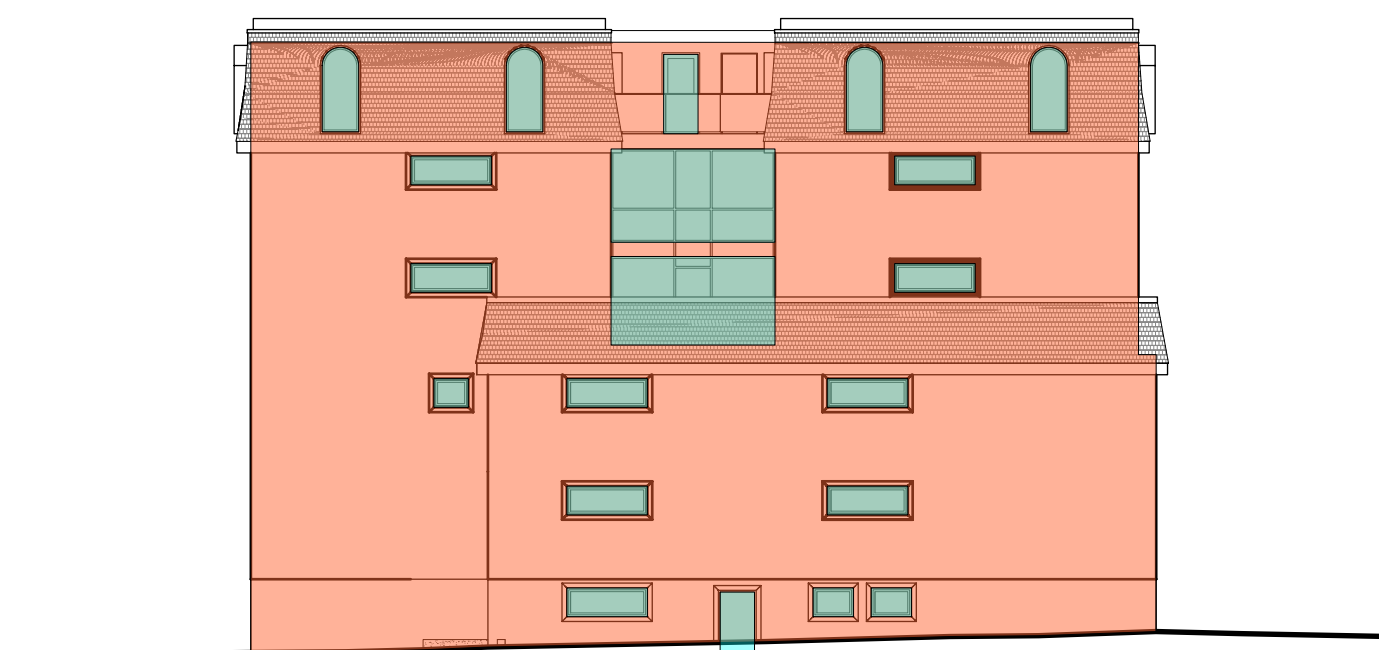
7 South Elevation Scale: 1:200 Table 3.2.3.1-D, BCBC DISTANCE TO PROPERTY LINE = 2.19 m AREA = 376.67 m 2 PROPOSED UNPROTECTED AREA = 49.77 m 2 UNPROTECTED OPENING ALLOWED 16%, 60.27 m 2 PROPOSED OPENING 13.21%
