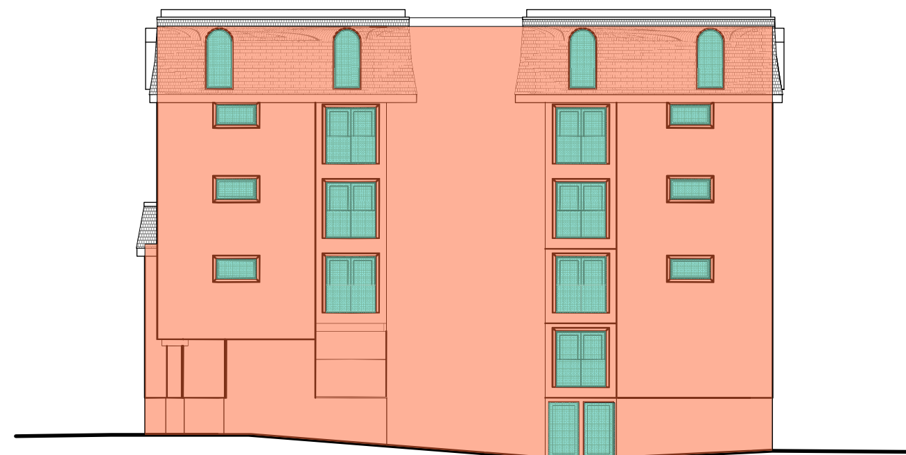
12 North Elevation Scale: 1:200 Table 3.2.3.1-D, BCBC DISTANCE TO PROPERTY LINE = 1.36 m AREA = 381.82 m² PROPOSED UNPROTECTED AREA = 48.8 m² UNPROTECTED OPENING ALLOWED 14%, 53.43 m² PROPOSED OPENING 12.79%
