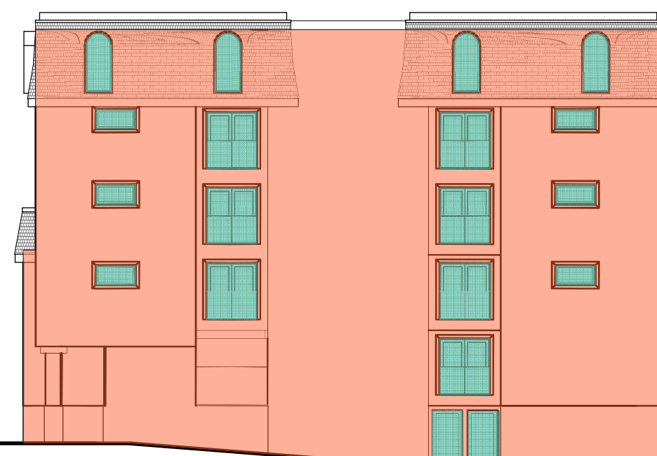
12 North Elevation Scale: 1:200 Table 3.2.3.1-D, BCBC DISTANCE TO PROPERTY LINE = 1.36 m AREA = 381.82 m 2 PROPOSED UNPROTECTED AREA = 48.8 m 2 UNPROTECTED OPENING ALLOWED 14%, 53.43 m 2 PROPOSED OPENING 12.79%
