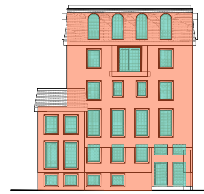
14 Front /East Elevation Scale: 1:200 Table 3.2.3.1-D, BCBC LIMITING DISTANCE = 10.08m AREA = 194.16 m 2 PROPOSED UNPROTECTED AREA = 54.17 m 2 UNPROTECTED OPENING ALLOWED 100%, 194.16 m 2 PROPOSED OPENING 27.90%
