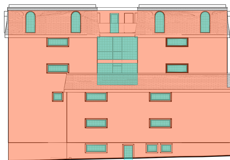
11 South Elevation Scale: 1:200 Table 3.2.3.1-D, BCBC DISTANCE TO PROPERTY LINE = 2.19 m AREA = 378.67 m 2 PROPOSED UNPROTECTED AREA = 49.77 m 2 UNPROTECTED OPENING ALLOWED 16%, 60.27 m 2 PROPOSED OPENING 13.21%
